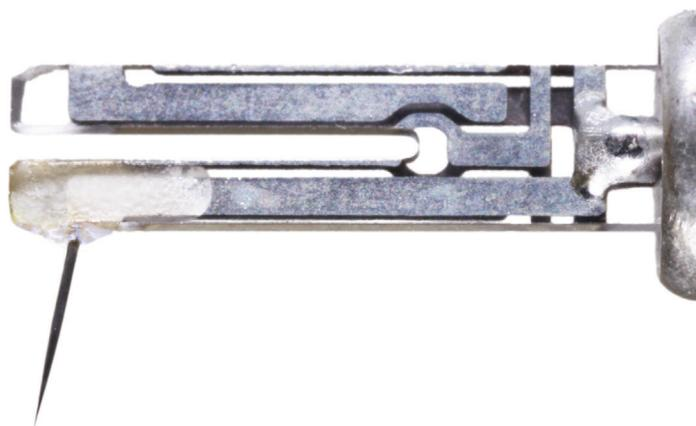
Figure 2. A quartz tuning fork with an etched tungsten tip.
