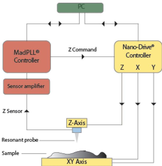
Figure 1. A schematic representation of an atomic force microscope, showing the phase lock loop controller, motion control hardware and resonant probe.
