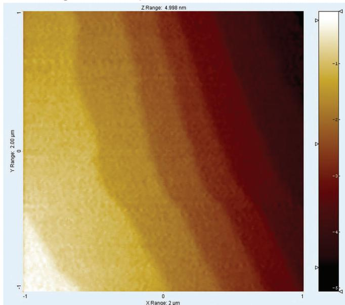
Figure 3. A two dimensional representation of Si (111) atomic steps measured by AFM. Each color shift represents a different atomic layer measurement. The average step height was calculated as 311pm with a standard deviation of 3pm in agreement with the accepted value of 312pm +/- 12pm.
