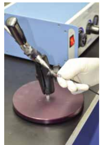
Fiber optic connector cleaning - close up.
