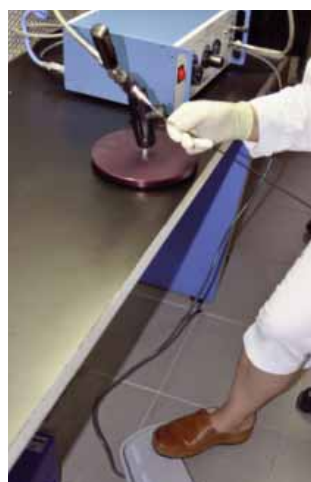
OZPEN cleaning high power patchcord.
