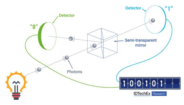
FIGURE 2. Schematic of a quantum random number generator (QRNG). Detecting the path of photons incident on a beam splitter creates a string of ones and zeroes with fundamental quantum randomness. Credit: IDTechEx
