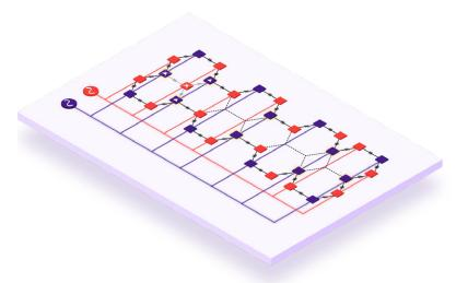
FIGURE 2. This schematic shows the proposed architecture addressing the wiring problem. Black and gray springs represent ZZ coupling between superconducting qubits. Purple and red squares represent two types of qubits, while purple and red lines represent the classical sources separately driving the qubits.
