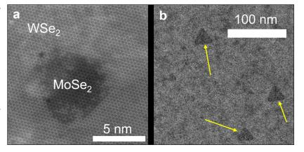
**FIGURE 1.** Atomically resolved TEM image of a MoSe<sub>2</sub> nanodot embedded in WSe<sub>2</sub> matrix (a); low magnification TEM image shows MoSe<sub>2</sub> nanodots (yellow arrows) dispersed in WSe<sub>2</sub> matrix (b).
