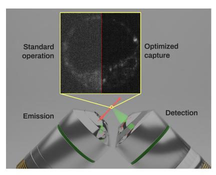
The setup of a light sheet microscope imaging a blastocyst embryo; a system of this type was used for analysis in the tutorial, and the optimization depicts the effects of confocal line scan mode.
