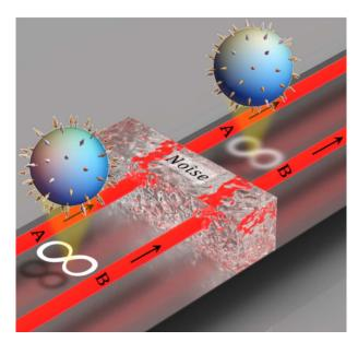
Two entangled photons, A and B, are engineered to be topological. After passing through a noisy real-world system, the entanglement decays but the topology remains intact. Credit: Pedro Ornelas
