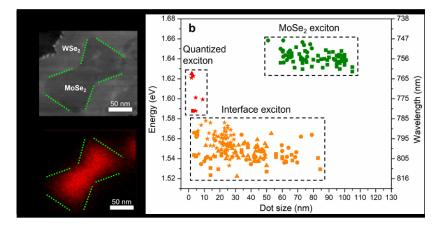
**FIGURE 3.** A TEM image of a MoSe<sub>2</sub> nanodot embedded inside WSe<sub>2</sub> (top left), where the contour of the nanodot is marked by dotted green lines; an artificially colored light emission intensity map of the same region shows the localized light emission from the nanodot (bottom left). A plot of energy of emitted light vs. the MoSe<sub>2</sub> nanodot size highlights the evidence of quantum confinement in nanodots under 10 nm in size (right).
