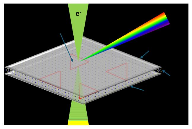
**FIGURE 2.** An illustration of our experimental setup: MoSe<sub>2</sub> nanodots, represented by red triangles, are embedded in WSe<sub>2</sub> matrix and encapsulated by hexagonal boron nitride (hBN) on top and bottom. An electron beam, shown in green, in a TEM is aimed at the heterostructure. The emitted light is collected by a detector.
