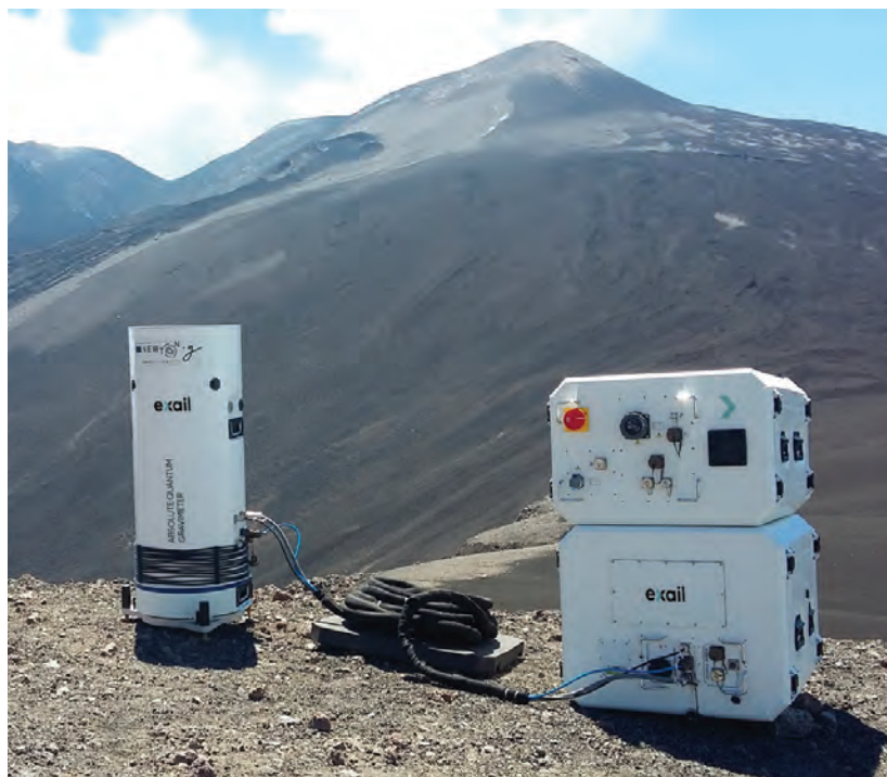
Deployed on the top of Mount Etna since 2020 by the Italian National Institute of Geophysics and Volcanology (INGV), Exail's Absolute Quantum Gravimeter has demonstrated its capability to detect minute gravity variations induced by magmatic activities. (Photo credit: Exail)
