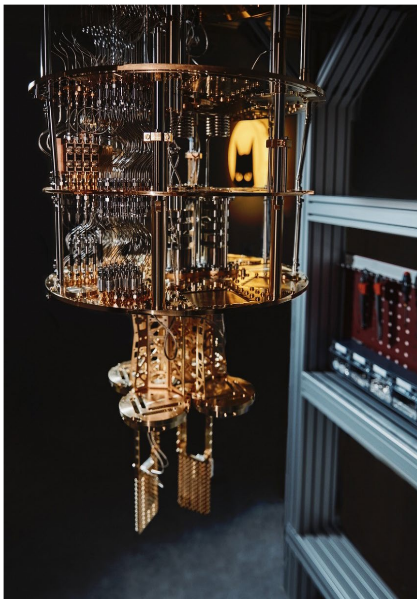
FIGURE 3. Alice & Bob's cryostat cools quantum memories down to 10 millikelvin.
