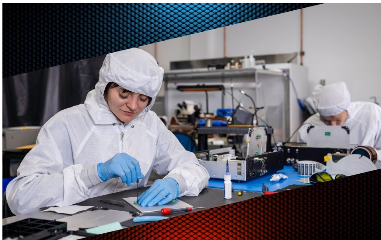
FIGURE 1. Vescent's team in the cleanroom assembling frequency combs. (Photo credits: Vescent)
