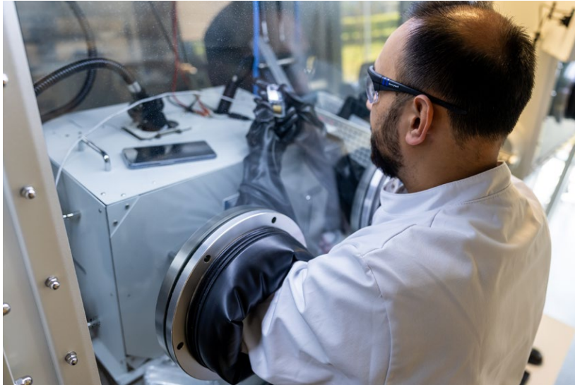
A scientist preparing a quantum-dot photodiode device for electrical measurement in a nitrogen-filled glove box.
