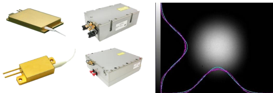
Figure 2.5 Focuslight FCM sources (left) and spot distribution (right)
