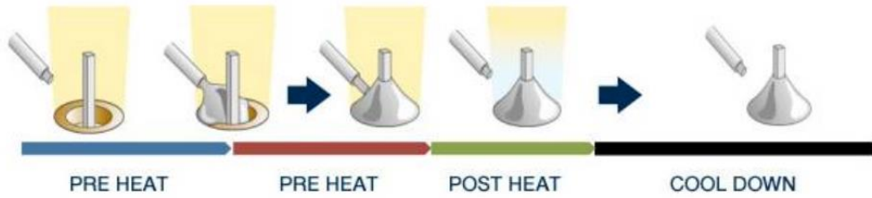
Figure 4.19 The process of the laser soldering
