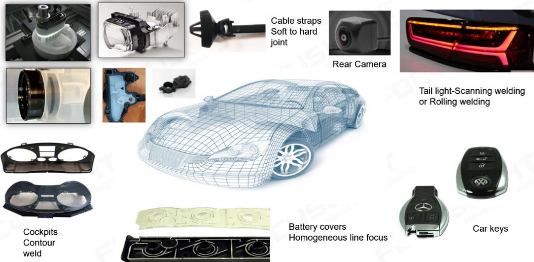
Figure 4.11 The laser plastic welding used in automotive car
