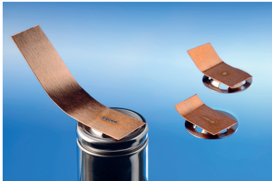
As part of the AiF project MikroPuls, Fraunhofer ILT is developing laser processes for the efficient contacting of battery cells (pictured: laser-welded copper connectors on cylindrical cells). (© Fraunhofer ILT, Aachen, Germany)
